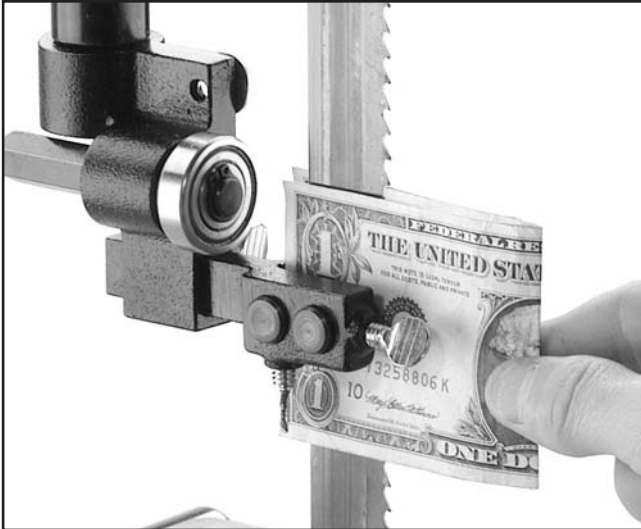
Figure 29. Single dollar thickness on each side of the blade.
